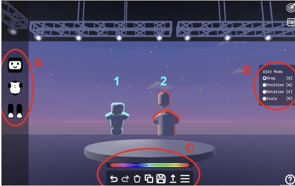
Fig. 2: A screenshot of the robot building tool with the part selection for drag and drop and the left side, a demonstration of an attached (1) and unattached part (2), the edit gestures on the right side, and the coloring and action menu on the bottom of the screen.
