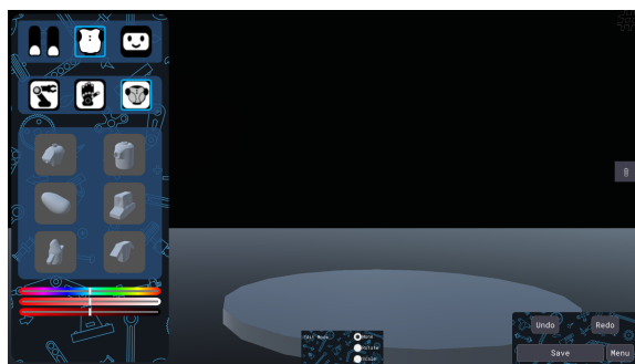
Fig. 1. The user interface for building robots on the Build-A-Bot platform prototype. On the left, the user can choose robot parts and colors. The parts can be dragged onto the turntable platform and positioned anywhere there. At the bottom, the user can choose to scale and rotate the parts. The user also has an undo, redo, and save option for their designs at the bottom right.
